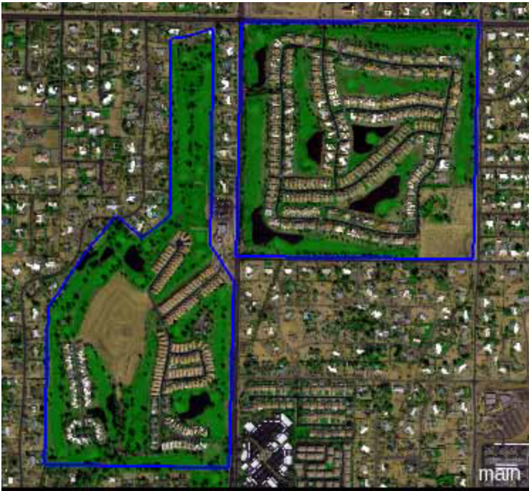
Figure 4: Image objects after executing the segmentation process. Only the outlines of the shapefile are represented.
